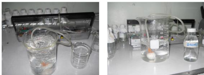
Figure 5. Actual Ozonation Process and Testing at Regional Water Analysis in Carmona, Cavite
